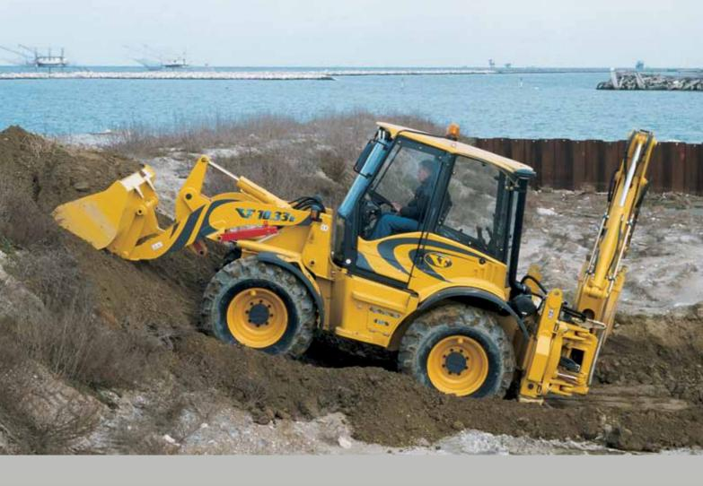
**VF 10.33B** is the only existing marriage between a 4x4x4 wheeled loader and a 6 meter excavating arm, the rigid backhoe loader guaranteeing the following:
